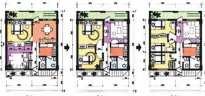
**MẶT BẰNG CĂN HỘ 4M (DT 56M<sup>2</sup>)**
